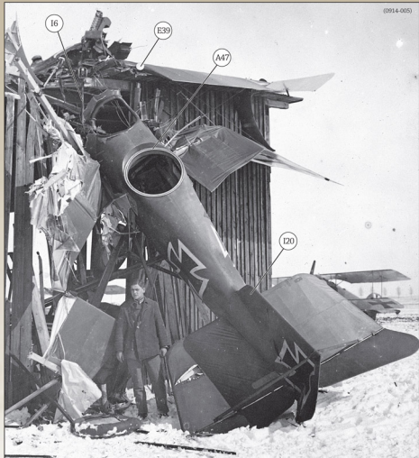
This final production Roland C.IIa "1" of Schusta 27b (Royal Bavarian Schutzstaffel 27, a protection squadron created from Kasta 36, Kagohl VI on 1 January 1917) has come to a sticky end after hitting a hanger at Puxieux, France in early 1917. Note the seam line running down the centerline of the fuselage! A bullet hole patch can be seen near the tip of the starboard horizontal tailplane, which is partially obscuring the Jasta 23b Albatros D.II in the background.
