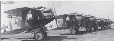
Three views of Kasta 2, Kagohl 1 showing a mix of late and final production Roland built C.IIa. Note the variety of personal markings and camouflage schemes.
