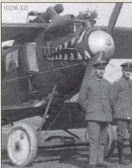
Undercarriage detail from the late production Roland C.IIa "White 2" seen on page 26. Note the claw brake and tyre valve access flap. (B6)
