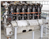
Early production 160hp Daimler-Mercedes D.III engine with the air pump (E48) at the rear as fitted in some Roland C.IIa, although most late production aircraft had the air pump fitted at the front (E5).
