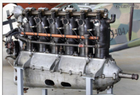
160hp Daimler-Mercedes D.III engine undergoing maintenance. The rocker arms and boxes (E8) and external water pipe (E3) have been removed.
