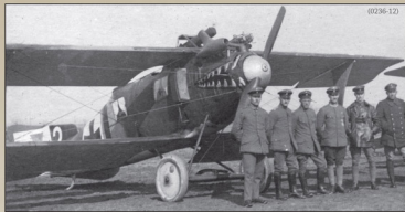
< Late production Roland built C.IIa "White 2" of Kasta 2, Kagohl 1 as seen on page 16. Note the protective cover over the IMG 08 "Spandau" machine gun, shark mouth markings and curtains painted in the windows.
